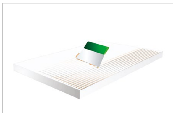
Application of acoustic adhesive D
