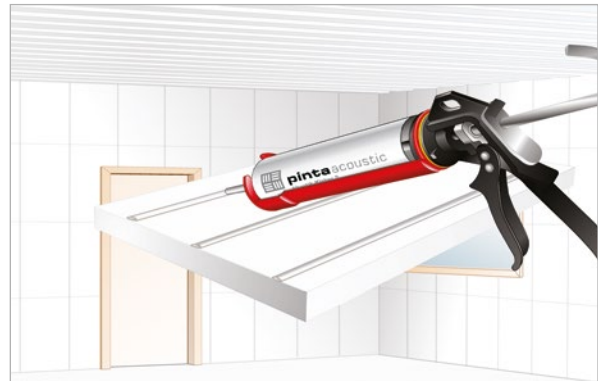
Application of acoustic adhesive S
