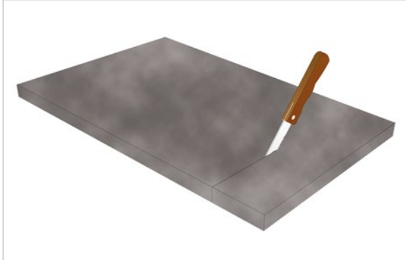
Cut absorber to required size
