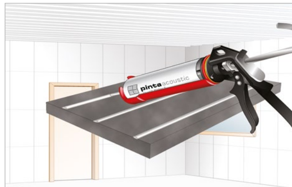
Apply acoustic adhesive
